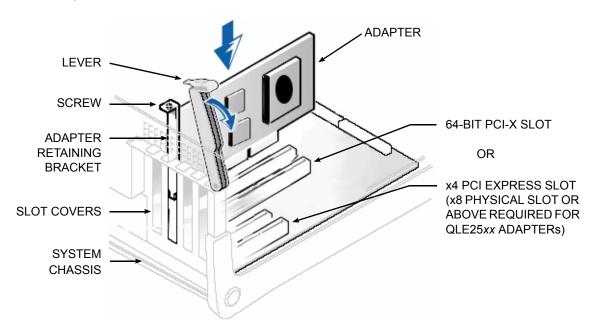
Figure 2-1 Installing the Adapter
